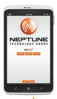
From here the user can select one of the three different functions of the app — RF Test. Data Log. or Off Cycle.
